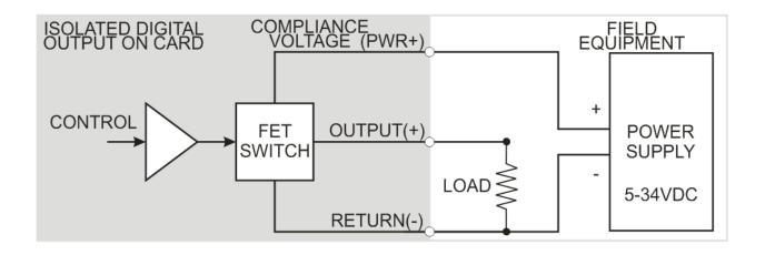
Figure 1-2: Simplified Output Connection Diagram
