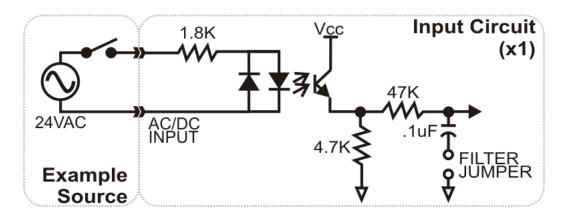
Figure 1-3: Simplified Input Connection Diagram
